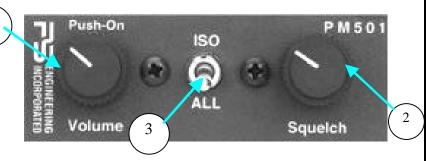
Turn the PM501 on pressing the volume control knob (left knob). This also engages the automatic fail-safe system.
